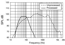
Processed: Before amplification, the audio signal is processed by the recommended high-pass, low-pass and EQ settings (see below).
